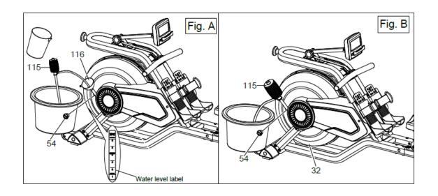
The amount of water in the Tank simulates the mass when moving an object in water. Changing the Water Level does not change the resistance, it simply changes the mass which the user is trying to move.
